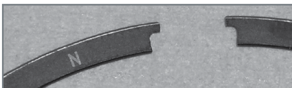
The letter marked on the piston rings.
