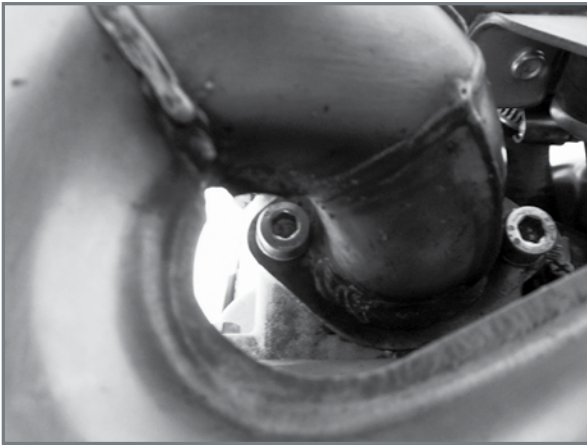
The two bolts of the exhaust manifold flange.
