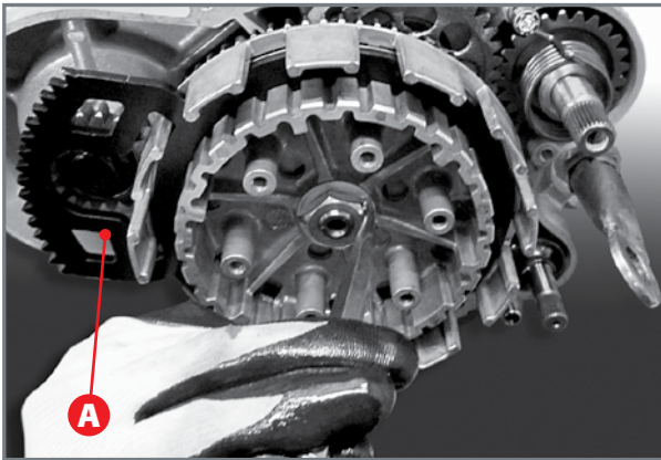
Opening the flaps of the safety washer.
