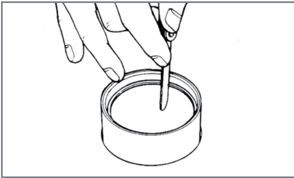
First verification of the piston rings.
