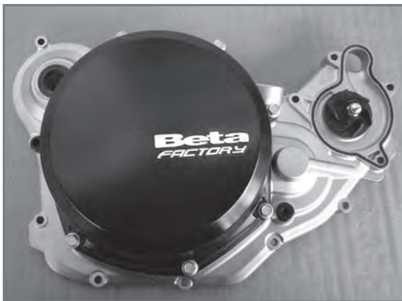
Complete internal clutch cove of water pump.
