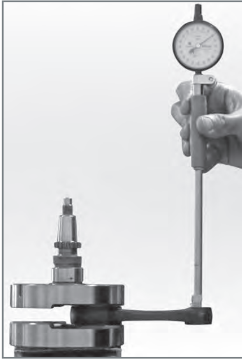
Bore meter verification of inside diameter of connecting rod foot.
