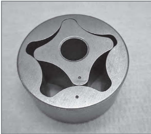
Low pressure pump: note the dot on the two rotors. The dot must face the inside of the engine.
