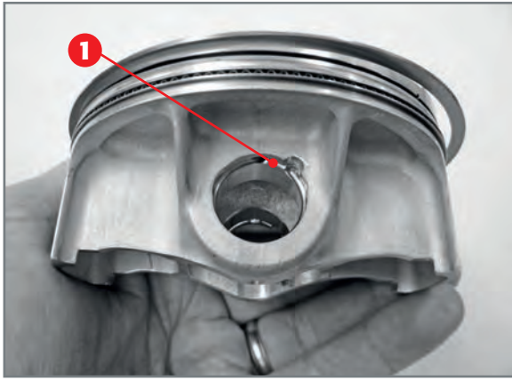
Application of circlip 1 to piston.
