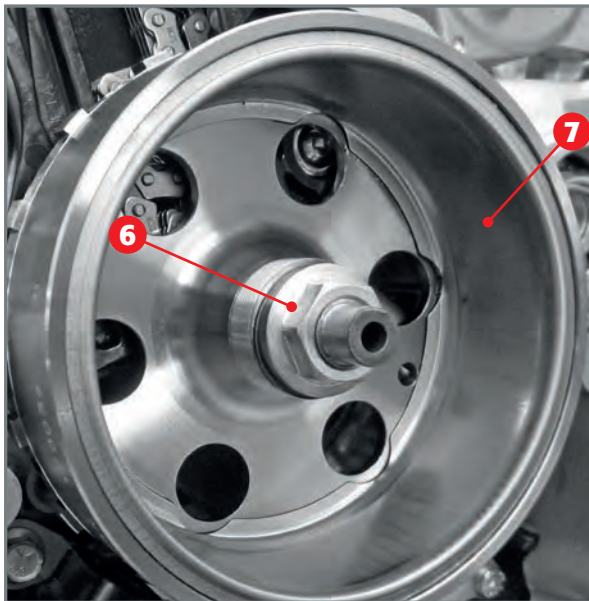
Nut 6 which fastens flywheel 7 to the crankshaft (injection version).
