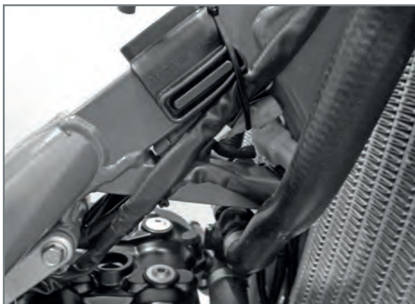
Electric connectors in the recess (injection versions).
