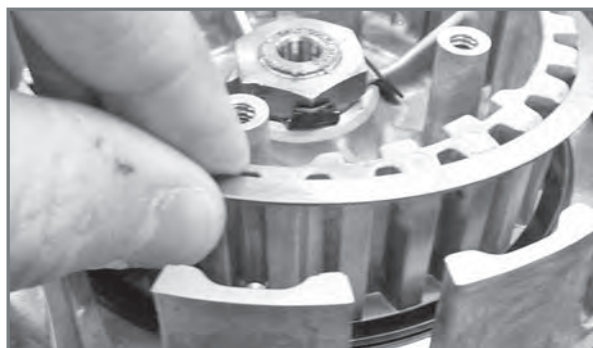
Removal of disc spring assembly.
