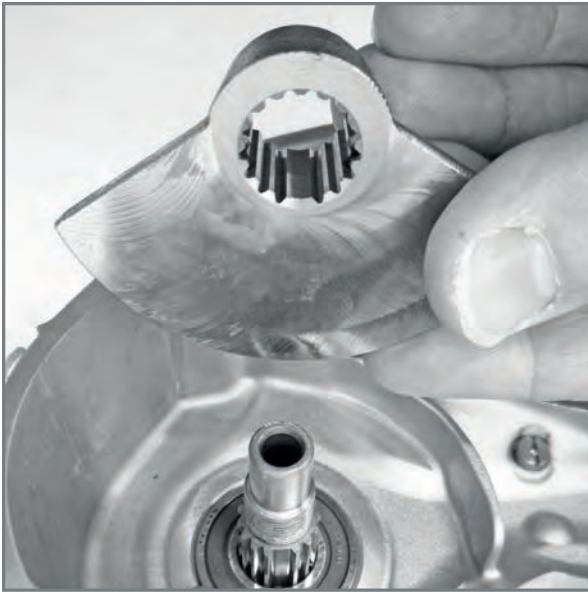
Coupling counterweight to countershaft.
