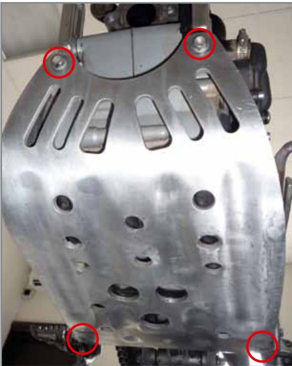
The four screws of the engine protection plate.
