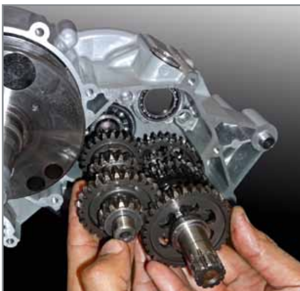
Inserting the gear in the left casing .
