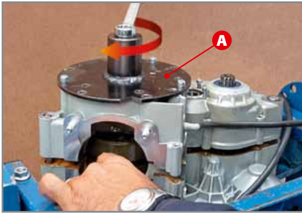
Decoupling the casings.
