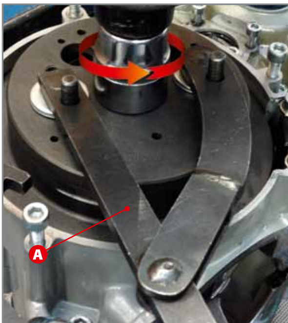
Blocking the flywheel with the universal tool.
