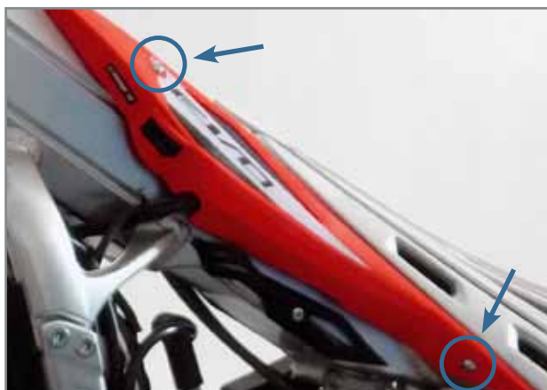
The screws that fasten the left side to the tank.
