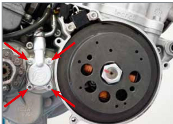
The four screws of the clutch actuator.
