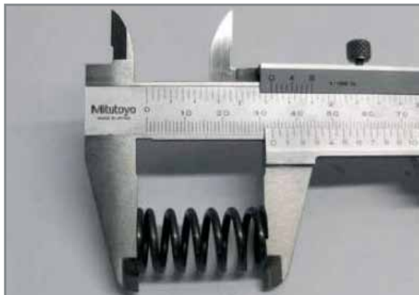
Measuring the length of the clutch springs.
