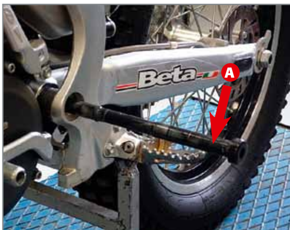
Swing arm bolt not being removed completely.
