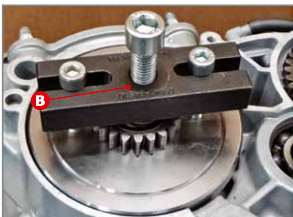
Disassembling the primary gear in 200 cc, 250 cc and 290 cc engines.
