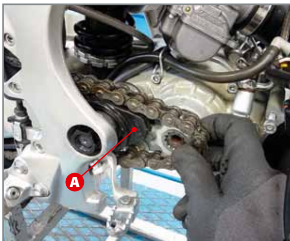
Inserting the pinion into the output shaft.
