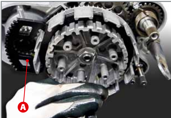
Opening the flaps of the safety washer.
