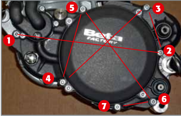
Layout of the screws on the internal cover of the clutch.
