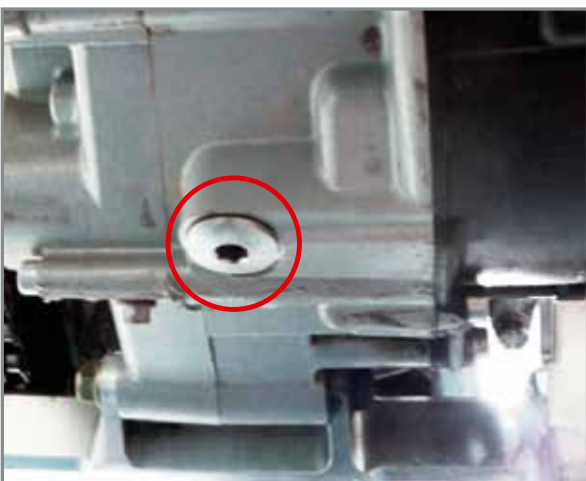
The plug where the transmission oil is drained from.
