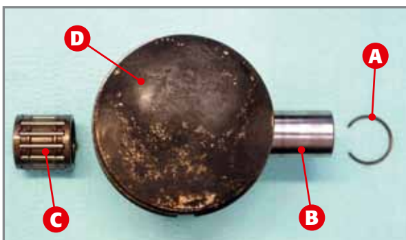
Complete piston: A) piston pin lock ring; B) piston pin; C) bearings assembly; D) piston.
