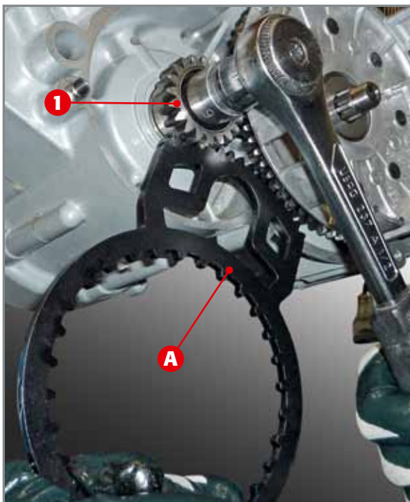
Disassembling the screw that blocks the primary gear to the motor shaft.
