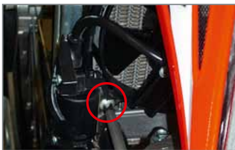
The screw that fastens the coil support to the radiator.
