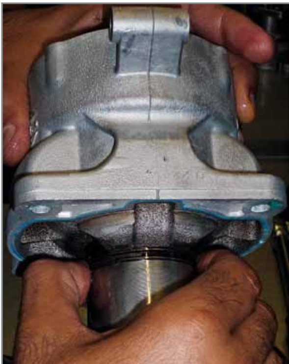
Inserting the piston into the cylinder.
