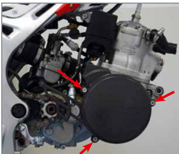
The three screws of the flywheel casing.
