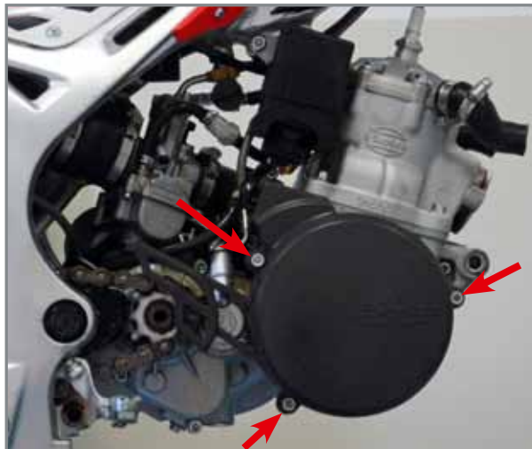
The three screws of the flywheel casing.
