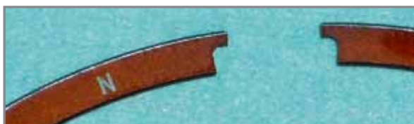
The letter marked on the piston rings.
