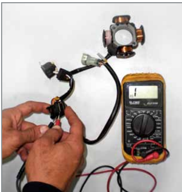
Verifying stator winding functionality.
