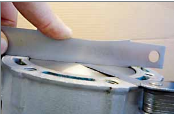
The tool touches the cylinder but don't touches the piston: Measure the clearance between piston and tool.
