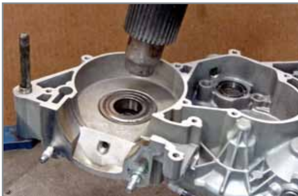
Heating the bearing.
