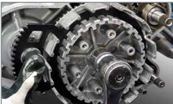
Disassembling the nut that blocks the clutch bell to the primary shaft.
