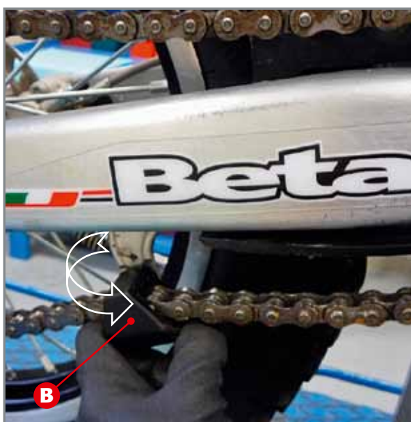
Rotating the chain tensioner
