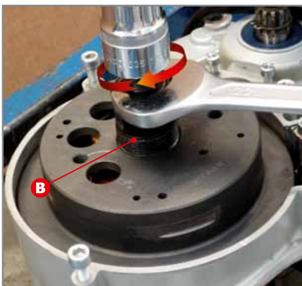
Decoupling the flywheel from the motor shaft by means of extractor B (code 1480210.000)
