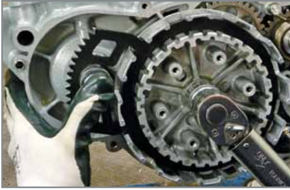
Tightening the nut that blocks the clutch bell to the primary shaft.
