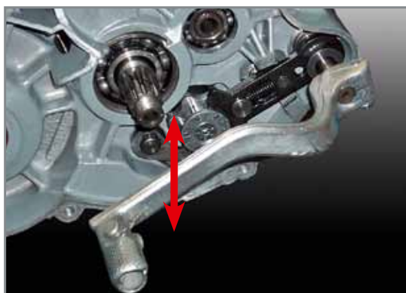
Verifying whether the gearbox unit functions properly.
