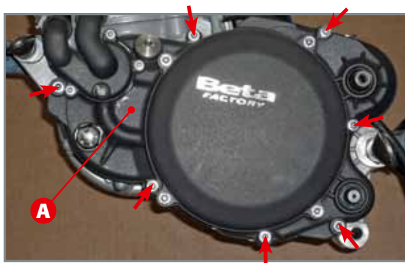
The seven screws that couple the internal cover of the clutch to the casing.
