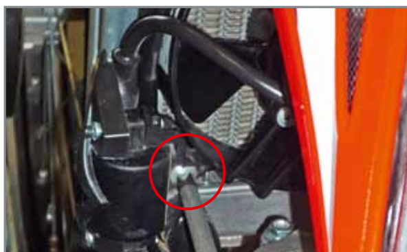
Reassembling the coil and support.
