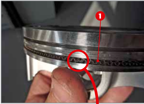
Application of central oil-scraper band.
