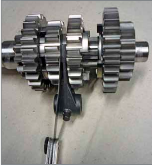
Checking wear of forks and gearwheels.
