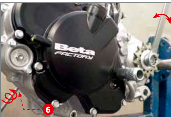
Blocking crankshaft at TDC. Note the blocking screw 6 and the movement set by the transmission shaft with the open-end spanner.
