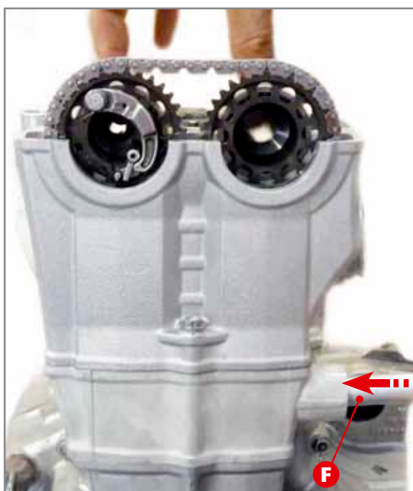
Phasing check. Note the pressure that the cylinder B exercises on the chain.
