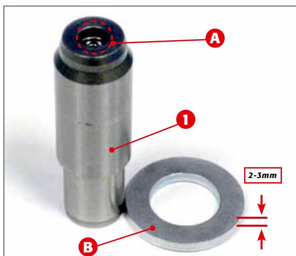
Preparation for hydraulic tensioner compression.
