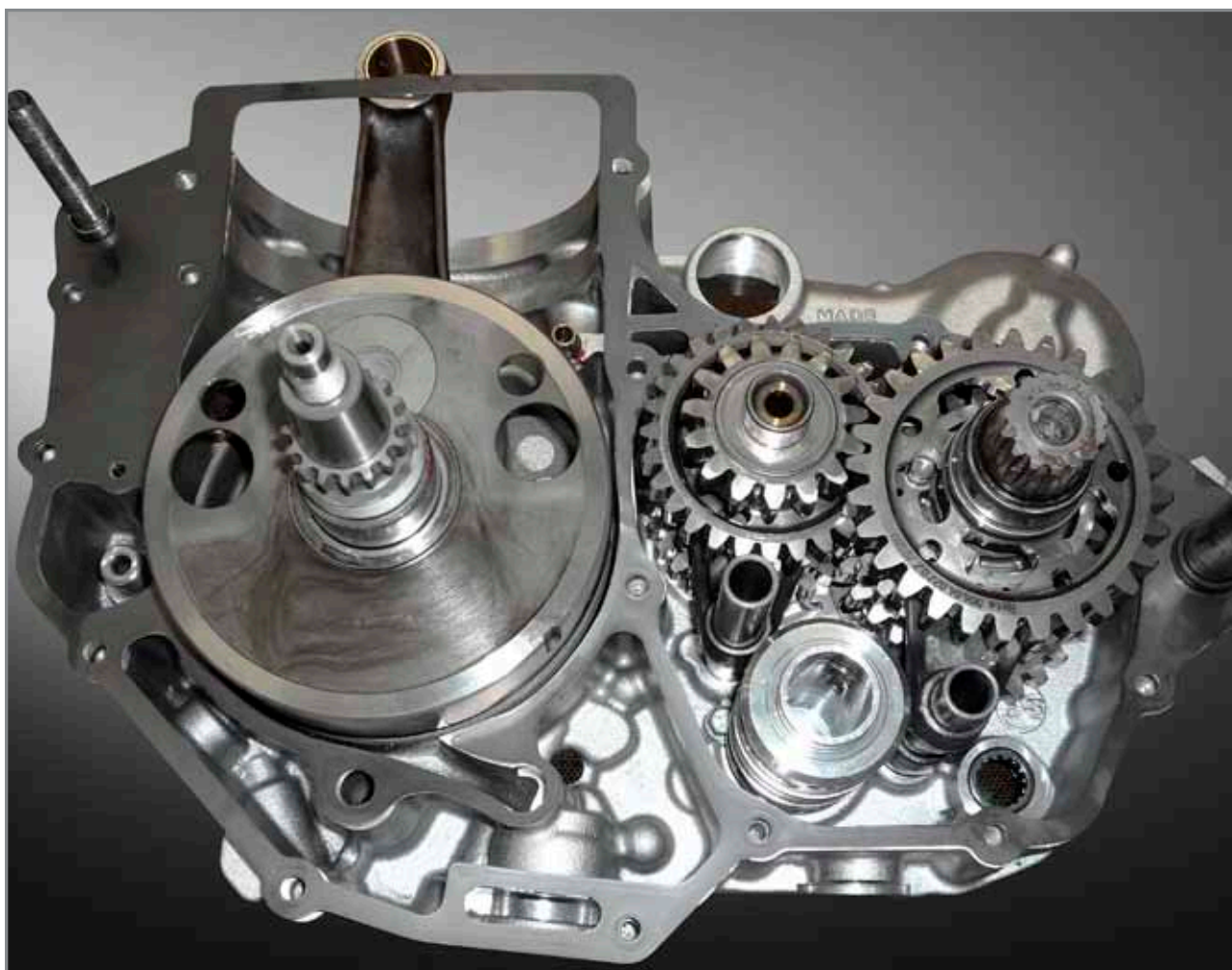
View inside the right crankcase with crankshaft, oil jets, gearbox shafts complete with gearwheels, internal gearshift and gasket.
