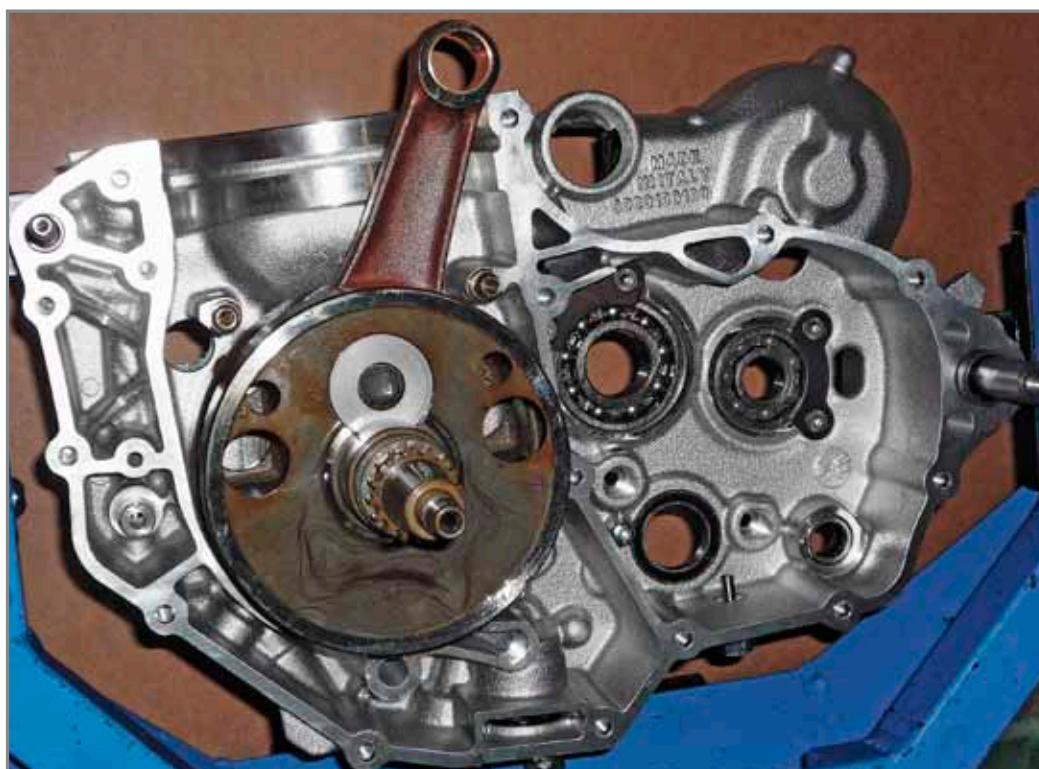
Insertion of crankshaft in right crankcase: note the position of the gear.
