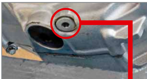
Location of pressure control valve.
