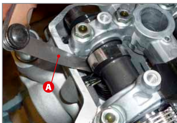
Checking valve play with thickness gauge.
