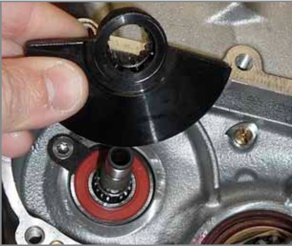
Coupling counterweight to countershaft.
