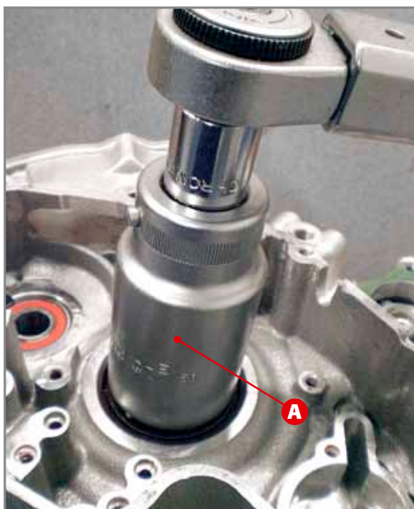
Removal of crankshaft nut with special socket wrench A.
