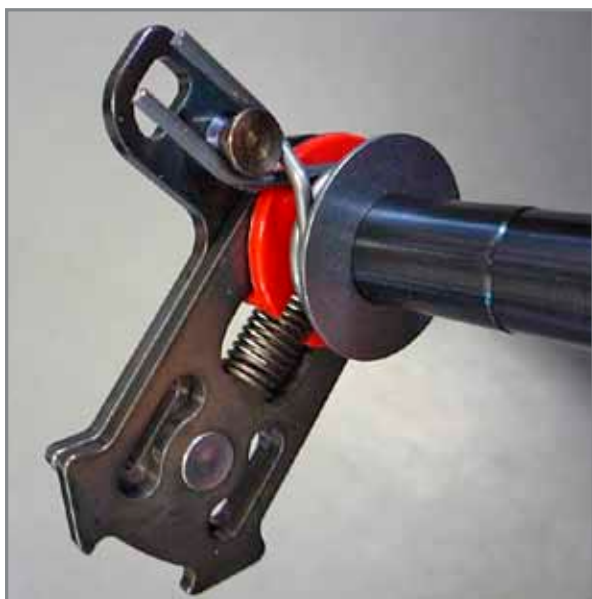
Gearshift drive shaft: note the positioning of the gearshift return spring.
