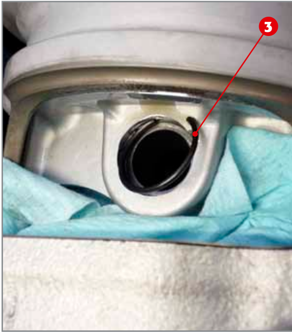
Application of circlip on piston coupled to the connecting rod.
