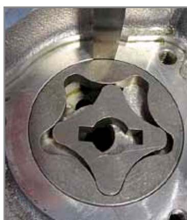
Assessment of radial play between external rotor and crankcase.
