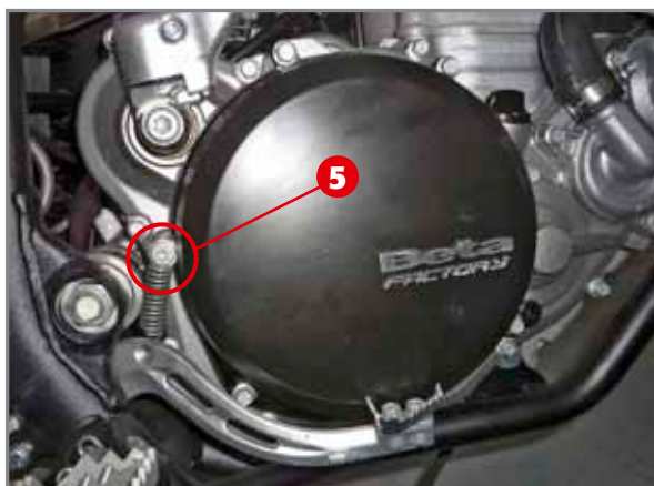
Detail of screw 5 to be applied with the engine coupled to a vehicle.
