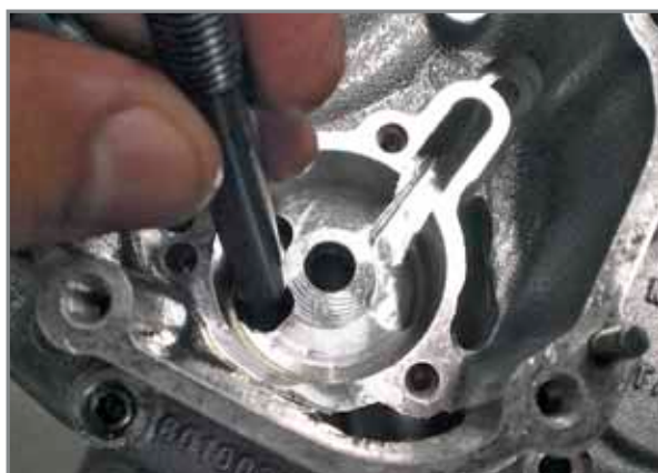
Removal from low pressure oil pump side.
