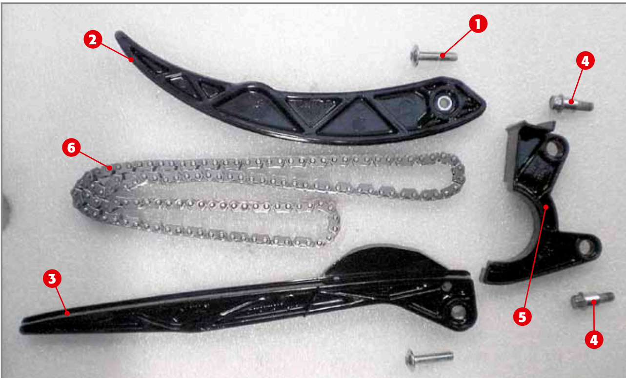
1) Two guide fixing screws; 2) Mobile guide; 3) Fixed guide; 4) Chain guard screws (complete with bushes); 5) Chain guard; 6) Timing chain.
