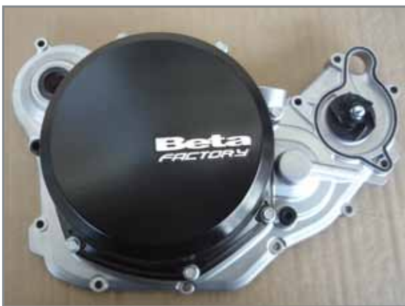
Complete internal clutch cove of water pump.
