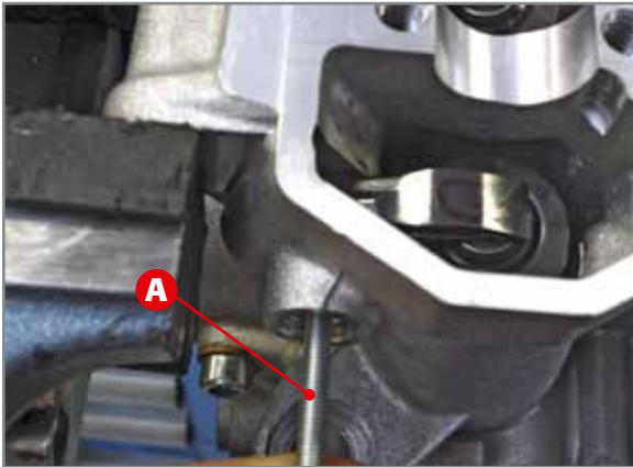
Application of M4 screw to allow pulling out the finger follower support shafts with your fingers.
