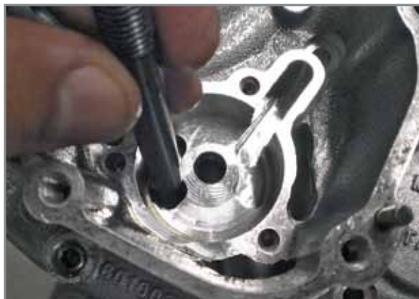
Removal from low pressure oil pump side.
