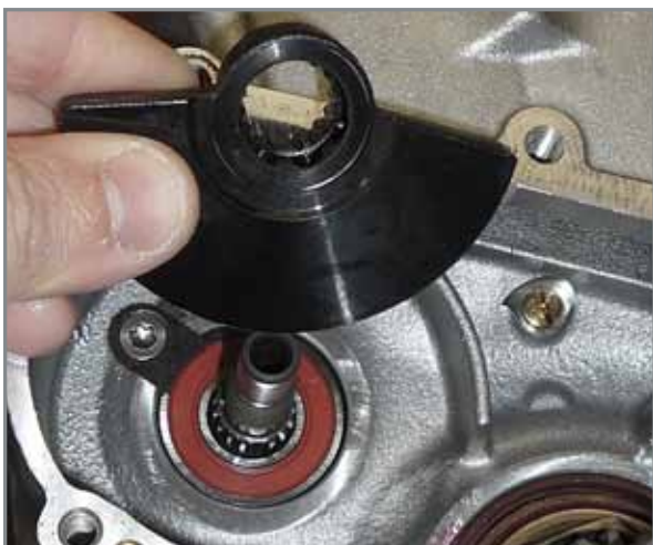
Coupling counterweight to countershaft.
