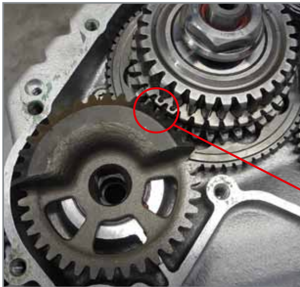
Coupling countershaft to crankcase.
