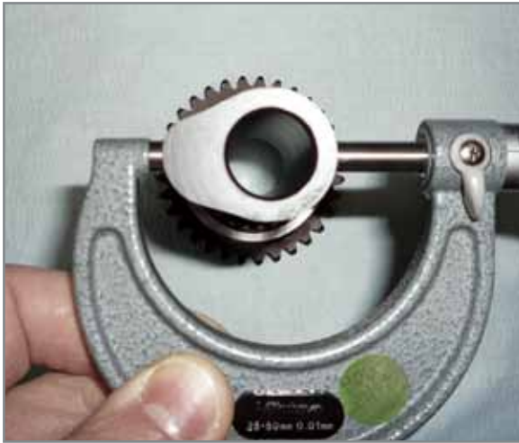
Cam height measurement.
