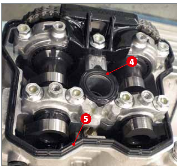
Spark plug gasket 4 and cylinder head cover gasket 5.
