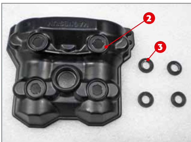
The cylinder head cover 2 and the four gaskets 3.
