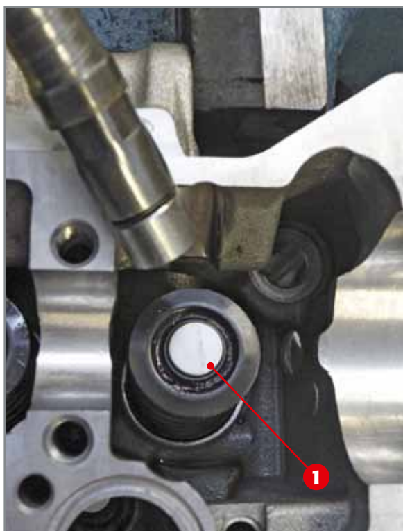
Removal of calibrated discs from seats.
