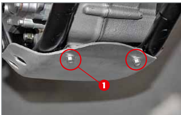
Back engine guard fixing screws.
