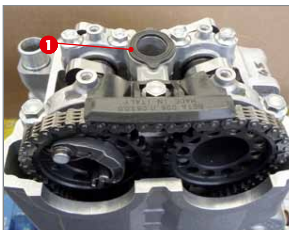
Application of spark plug gasket.
