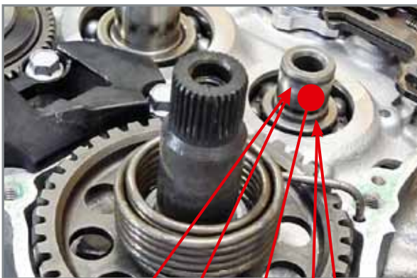
Insertion of kickstart return spring.
