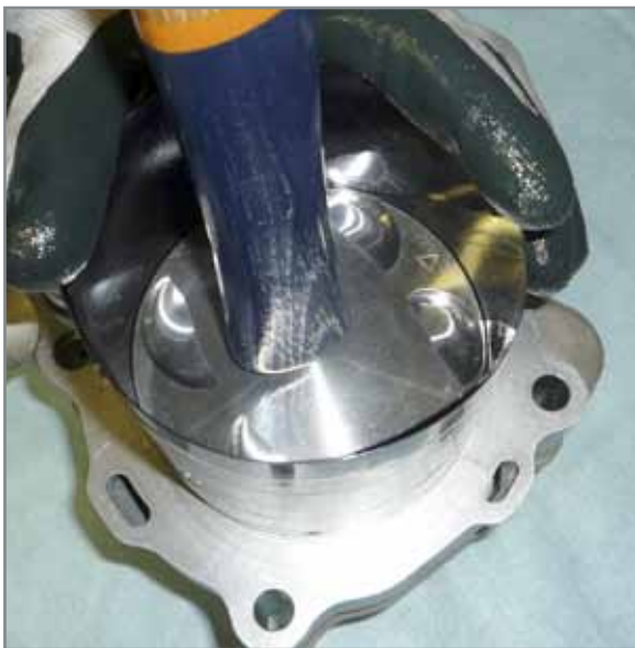
Insertion of piston in cylinder.
