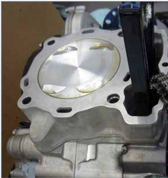
Coupling cylinder to crankcase.
