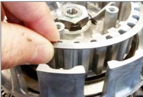
Removal of disc spring assembly.
