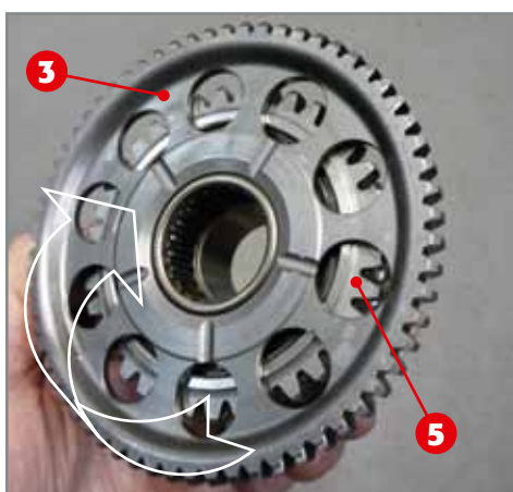
Main gear complete with free wheel coupled to ignition gear.
