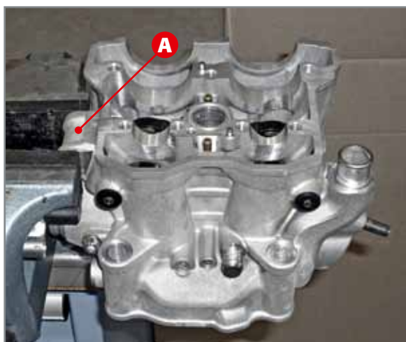
Blocking cylinder head on vice.
