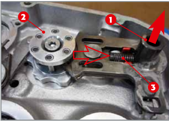
Disassembly of drive shaft.
