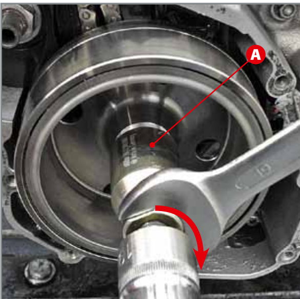
Removal of ignition flywheel with relevant extractor A.
