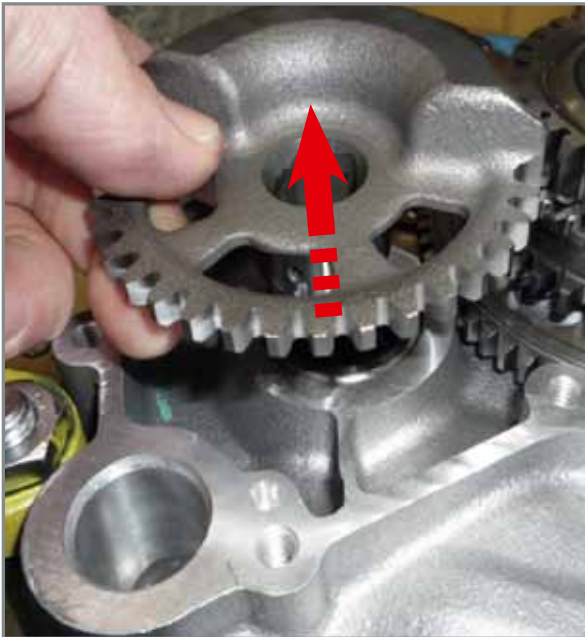
Extraction of countershaft.
