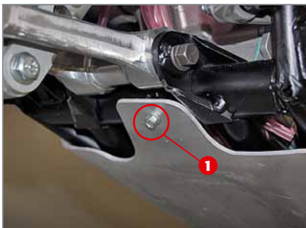
Front engine guard fixing screw.
