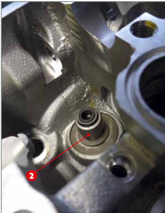
Insertion of valve stem seal.
