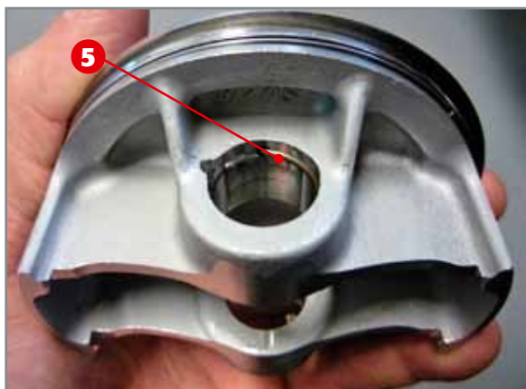
Application of circlip 5 to piston.
