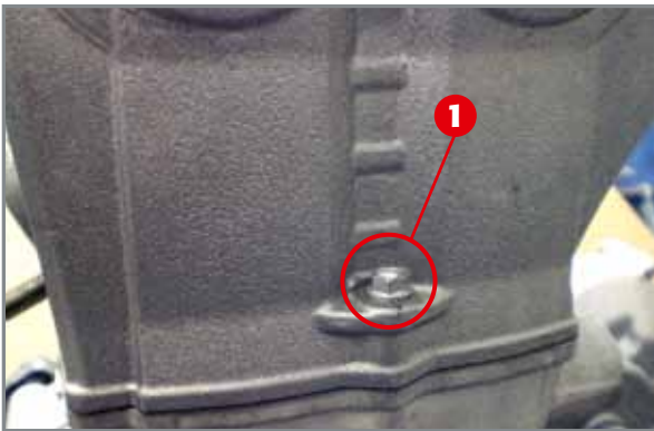
Chain-side head fixing screw.
