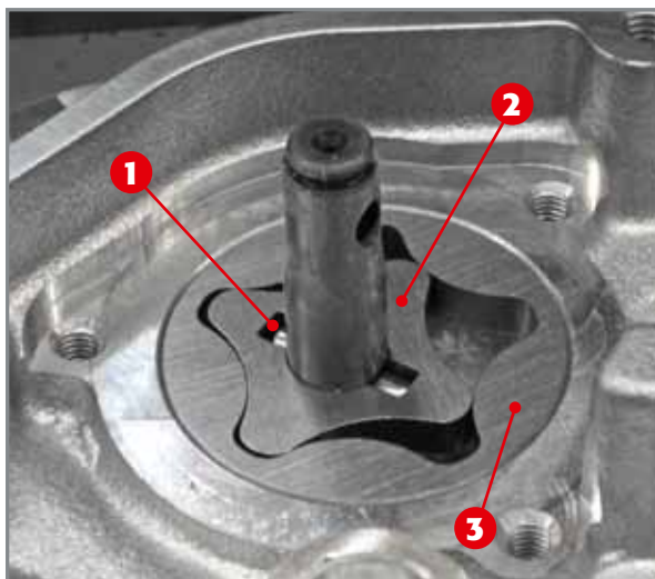
Coupling high-pressure pump rotors to drive shaft.
