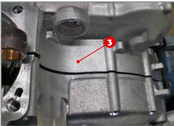
Detaching crankcase halves.
