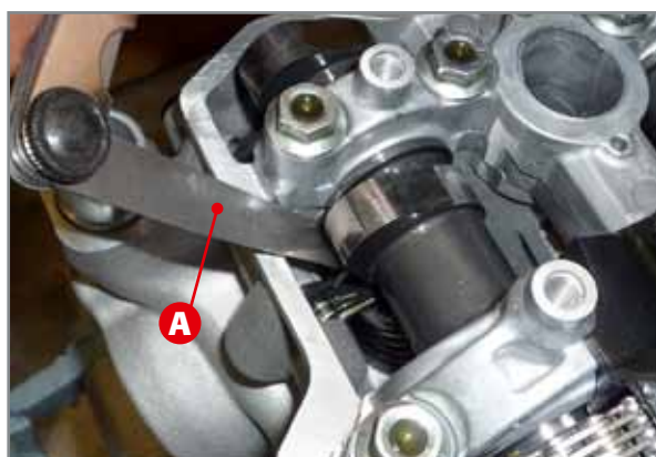
Checking valve play with thickness gauge.
