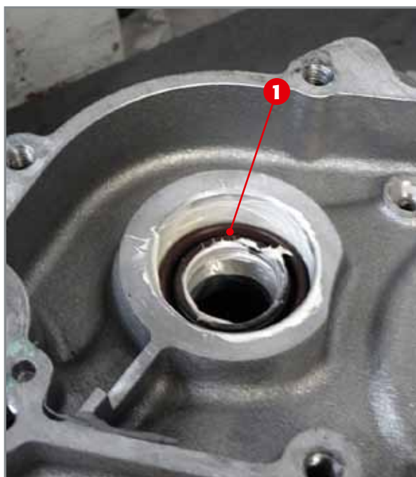
Application of oil seal 1.
