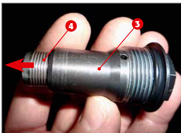
Tensioner support complete with piston.
