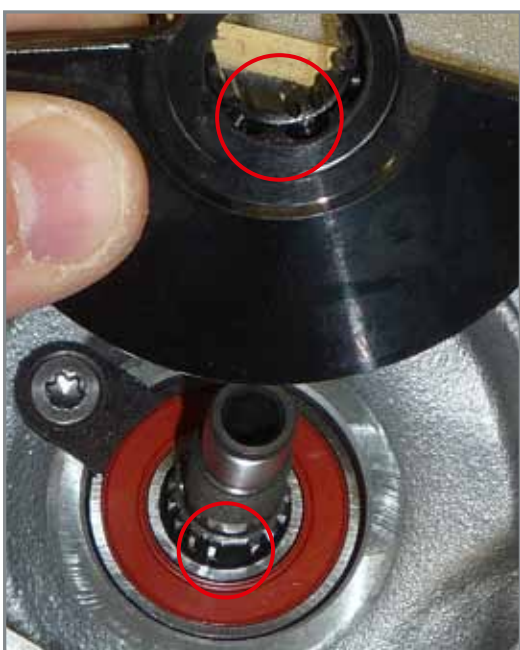
Detail of grooved profiles for coupling.
