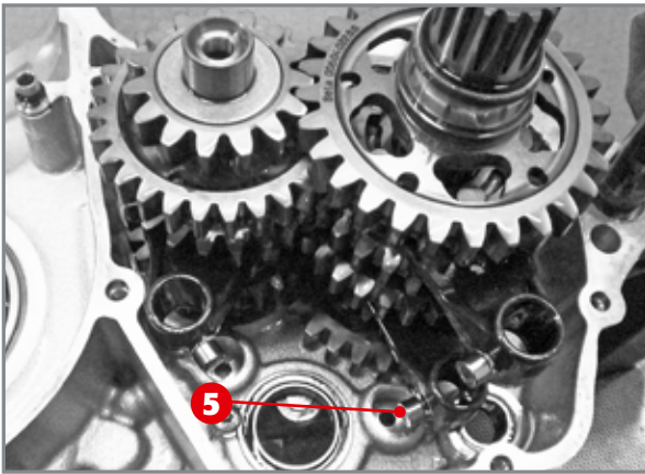
Extraction of forks from gearbox unit.
