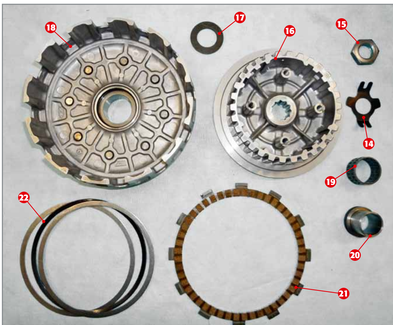
Safety washer 14 , nut 15 , inner hub 16 , washer 17 , basket 18 , roller cage 19 and bush 20 , special fiction disc 21 , judder spring 22 .
