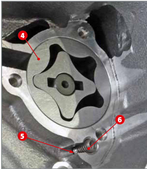
Complete low pressure pump coupled to the crankcase.
