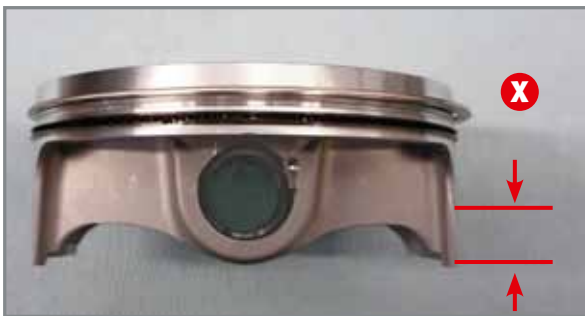
Quota at which to measure the outside diameter of the piston.
