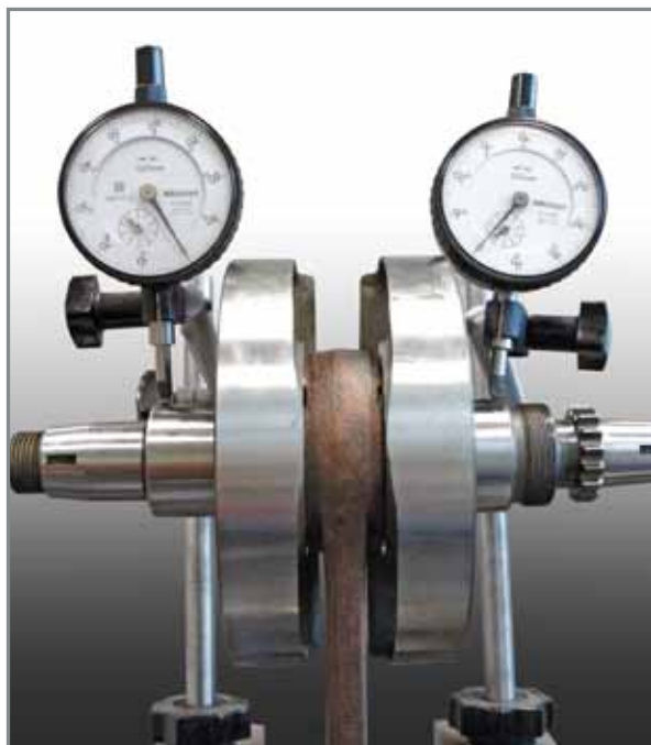
Deflection/Off-centring of crankshaft.
