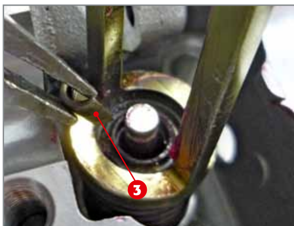
Spring compression, half-cones insertion. Note the application of grease on the upper part of the stem.
