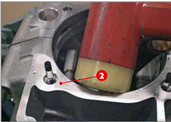
Disassembly of crankcase.
