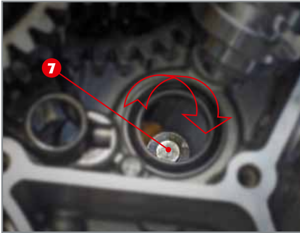
Insertion of desmodromic device in specific bearing. Note the rotation of the stop lever.
