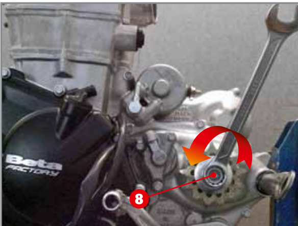
Rotation of transmission shaft.
