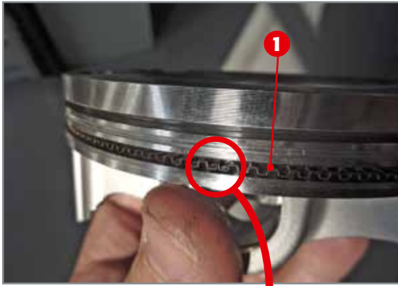
Application of central oil-scraper band.
