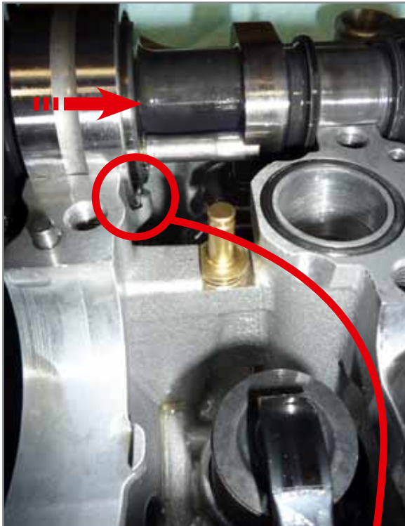
Positioning camshaft bearing.
