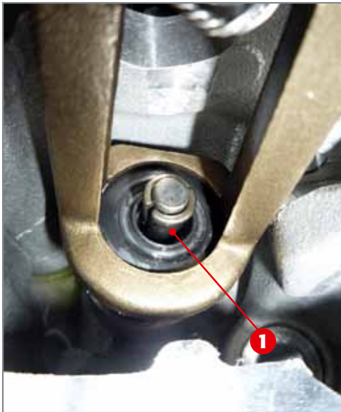
Extraction of half-cones.
