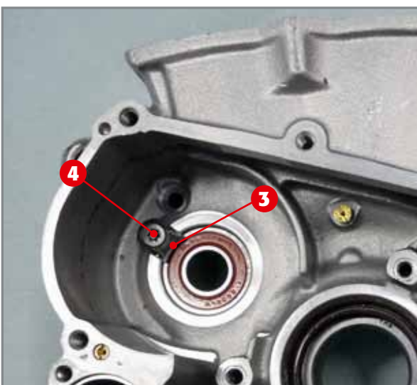
Outside safety plate of left crankshaft half counter- shaft.
