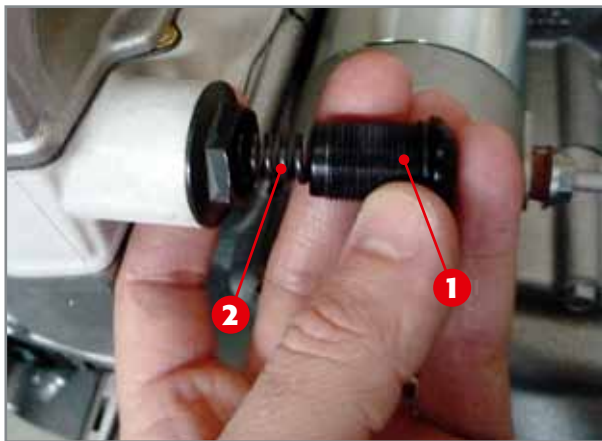
Cap and spring removal.
