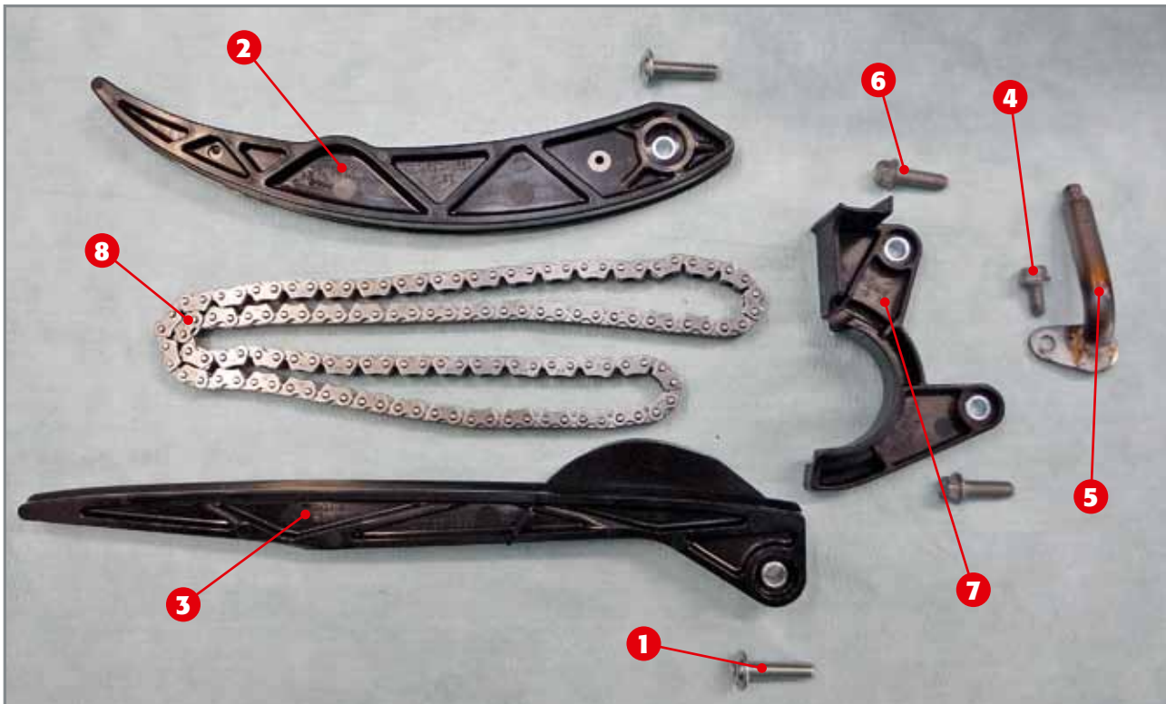
Two pad fixings screws 1 ; mobile pad 2 ; fixed pad 3 ; oil jet fixing screw 4 ; oil jet 5 ; chain guard fixings screws 6 ; chain guard 7 ; timing chain 8 .
