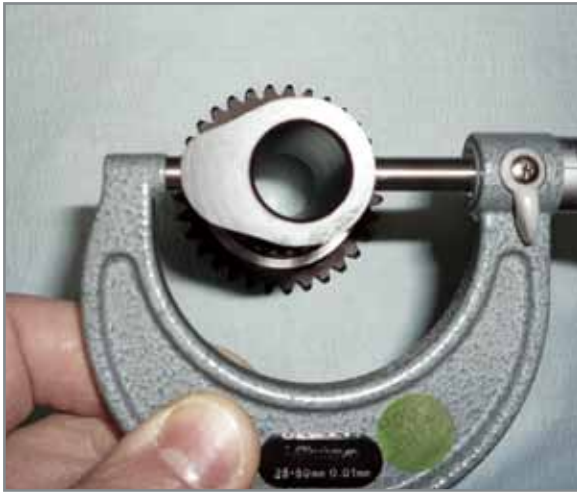
Cam height measurement.
