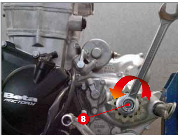
Rotation of transmission shaft.
