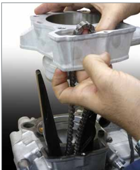
Passage of chain in cylinder.
