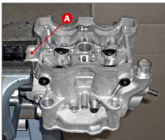
Blocking cylinder head on vice.
