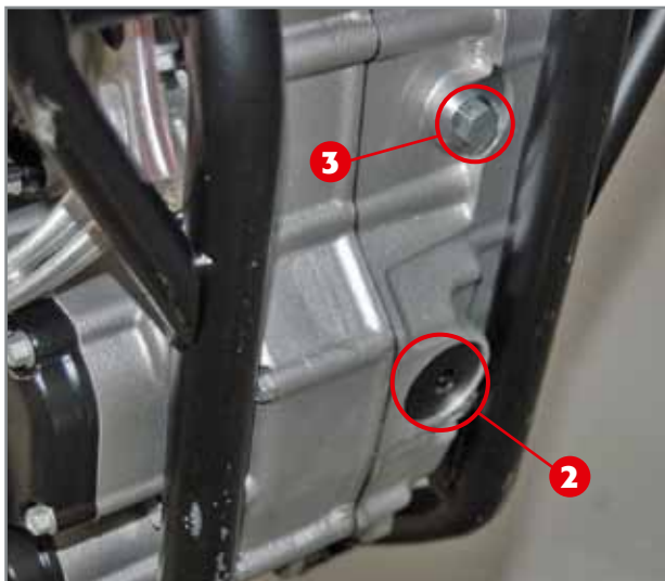
Screw 2 for draining motor oil and 3 for draining gear oil.
