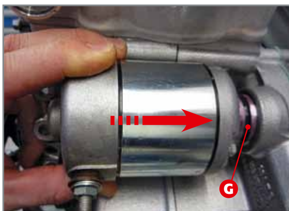
Insertion of start motor in crankcase half. Note zone G to be greased.
