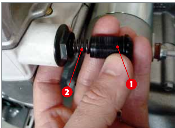
Cap and spring removal.
