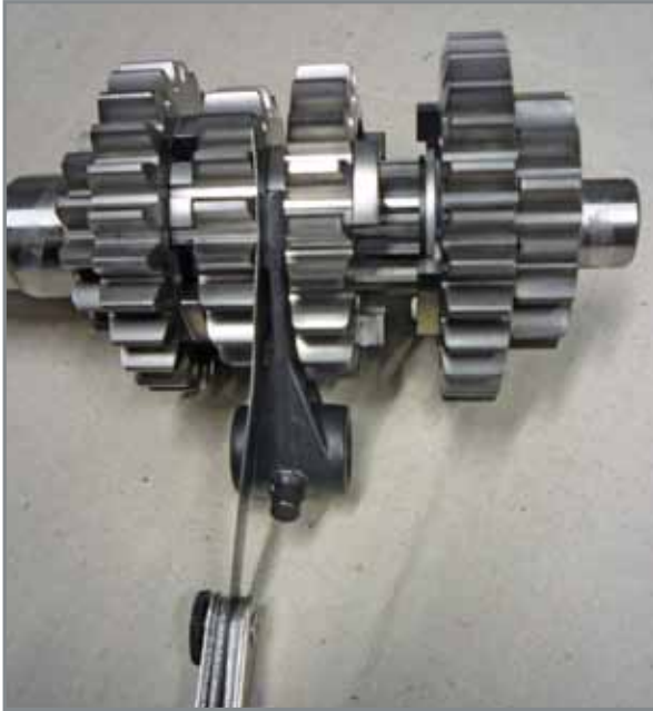
Checking wear of forks and gearwheels.
