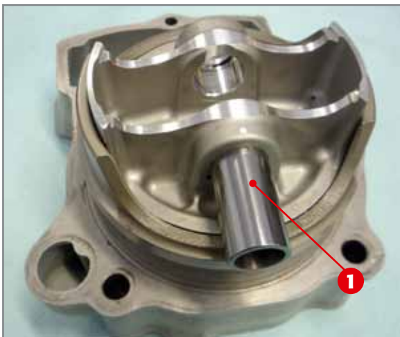
Application of pin bolt to piston.
