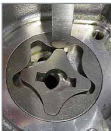
Assessment of radial play between and internal and external rotor.
