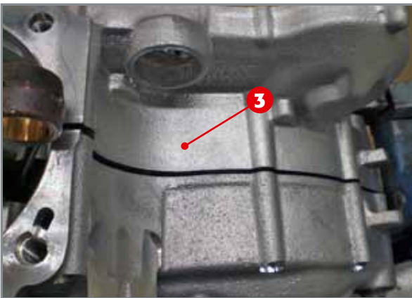
Detaching crankcase halves.
