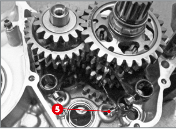
Extraction of forks from gearbox unit.
