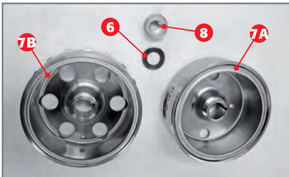
Flywheel 7a (carburettor version), 7b (injection version), nut 6 and special washer 8.
