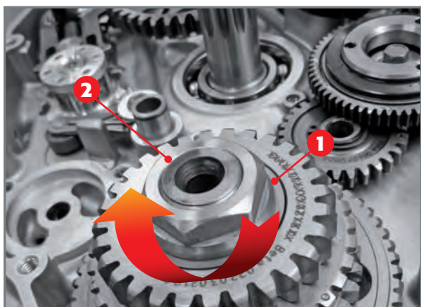
Primary gear 1 and relative nut 2.
