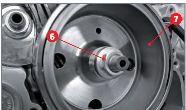
Nut 6 which fastens flywheel 7 to the crankshaft (carburettor version).
