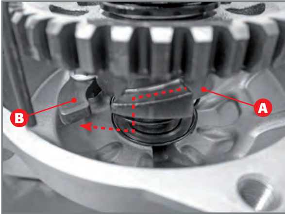
Positioning of sleeve A below ramp B.
