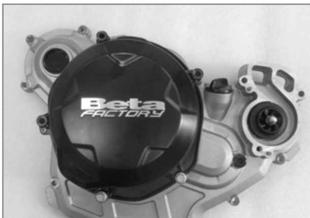
Inner clutch cover with water pump.
