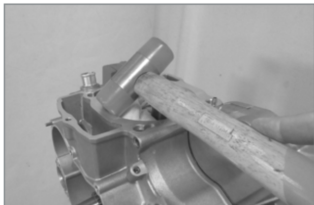
Disassembly of crankcase.
